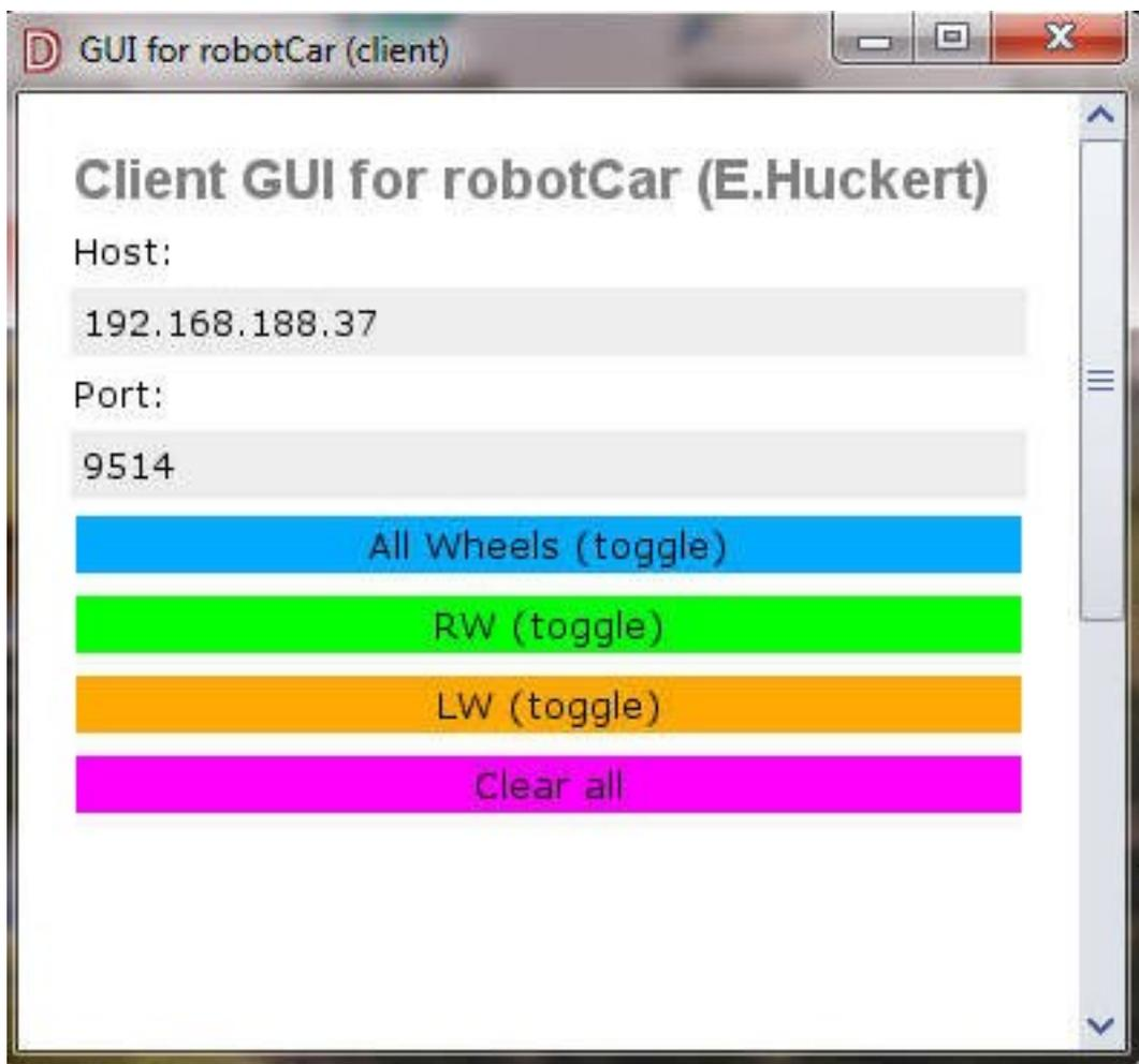
The 4 buttons are used to output strings as described above. The two entry fields can be used to enter the **IP address** and the **port number** needed for UDP.
