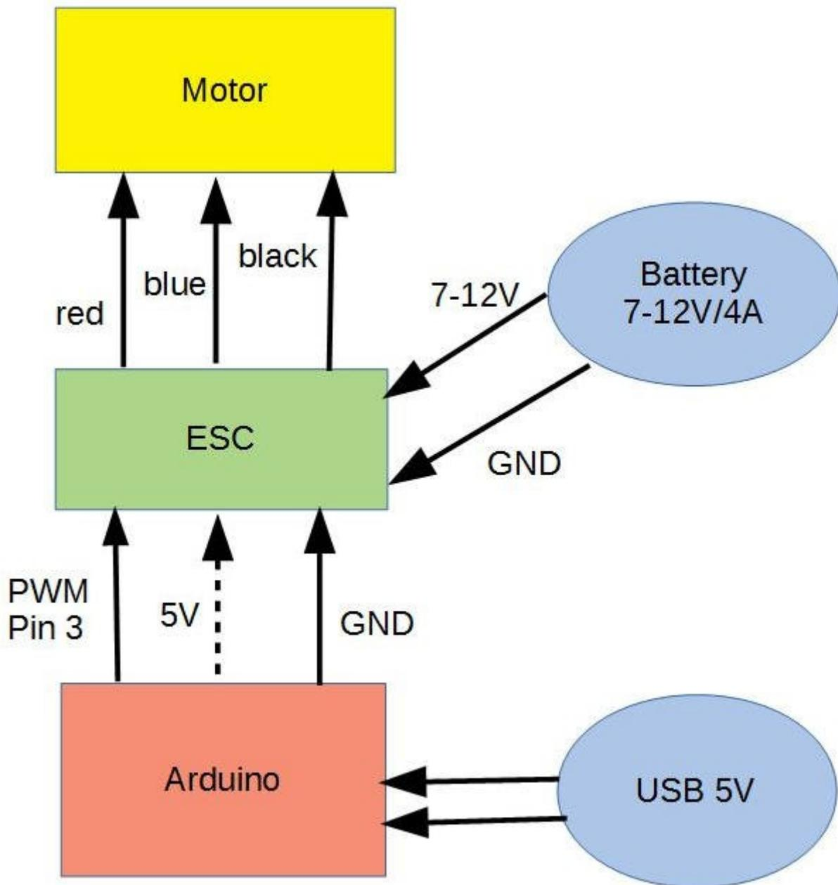
Note: the 5V connection from Arduino to ESC is not needed (dotted line). If you use other PWM pins on the Arduino be sure that they are speed-compatible with you ESC (490 or 980 Khz). The colours of the cables may be different if other components are used.
